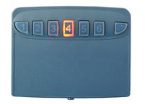
A small Pager unit worn by the Carer. When the Pager receives a signal it illuminates one of the numbered keys and beeps or discreetly vibrates to alert the carer of an event. The units internal battery is recharged each night in the Care Call trickle charger.
