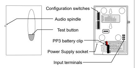
1. Move Key 15 to the right. Connect a 9V Alkaline PP3 to the battery clip.
