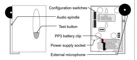
1 Move Key 15 to the right. Connect a 9V Alkaline PP3 to the battery clip.
