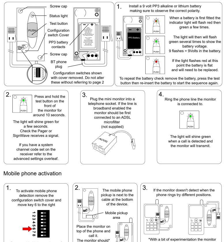
Press and hold the test button for 10 seconds to transmit the monitor
