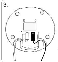
Connect the mains adaptor to the SignWave base and plug adaptor into a 13 Amp mains socket.
