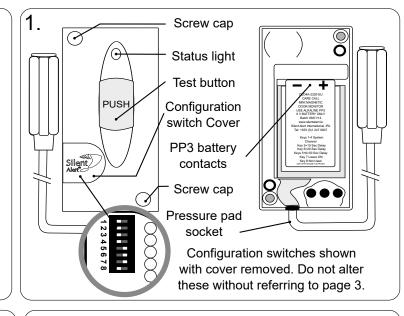
Install a 9 volt PP3 alkaline or lithium battery making sure to observe the correct polarity.
