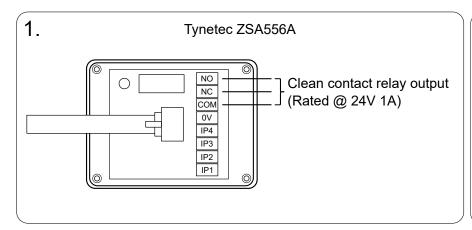
Connect a suitable length of twin core low voltage cable to terminals NO & COM of the Tynetec unit (shown here in grey and black).
