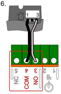
Connect a suitable length of twin core low voltage cable to terminals 3 & 4 of the Tunstall unit (shown here in grey and black).
