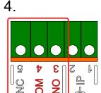
The hardwired output in Vi+ home unit provides common (COM), normally closed (NC) and normally open (NO) contacts.
