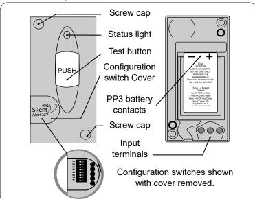
1. Install a 9 volt PP3 alkaline or lithium battery making sure to observe the correct polarity.
