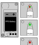
When a battery is first fitted the indicator light will flash red then green a few times.
