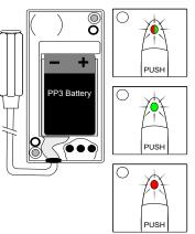
When a battery is first fitted the indicator light will flash red then green a few times.
