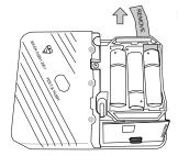
Remove the battery tab by pulling out and away from the unit.
