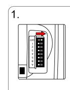
Move the ON/OFF switch to the on position (to the right, away from off).
