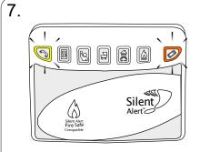
If the low battery sequence alternates with another event key, that monitor has a low battery.
