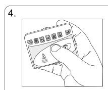
To re-set the Pager and stop the vibration, press and hold the key that is lit.
