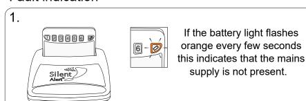
Check the Power Supply is firmly connected to the unit.
