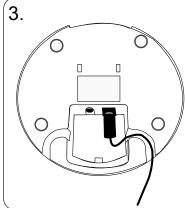
Connect the mains adaptor to the SignWave base and plug adaptor into a 13 Amp mains socket.
