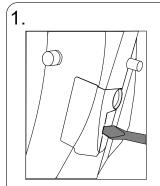
Insert a small flat blade screwdriver into the slot on the front cover.
