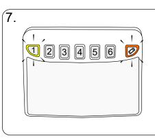
If the low battery sequence alternates with another zone key the monitor configured to send that zone has a low battery. Replace the Monitor battery and transmit to test.
