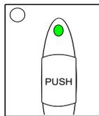
After the flashing red/green startup sequence the light will shine constant green.
