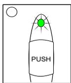
To set the zone number, briefly press the test button at the desired number of flashes.
