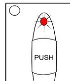
Press and release the test button whilst the light is green. The light will flash red once, twice then three times and so on up to twelve.
