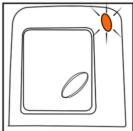
If the light shines orange when the button is pressed the internal battery is low and should be replaced (see step 3).
