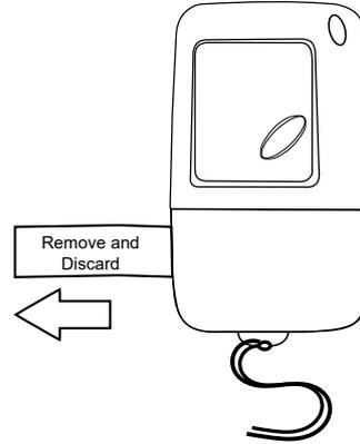
To activate the unit simply remove the paper tab by pulling it gently away from the unit.
