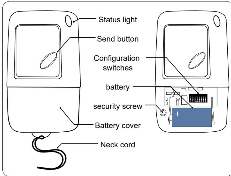
1. A battery is already installed in the Keyfob.
