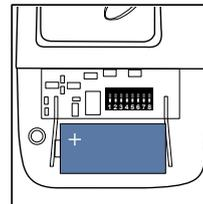
Replace with a 6V lithium battery (2CR1/3N OR PX28L)
