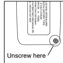
When the battery needs replacing remove the screw from the rear of the unit.
