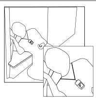
For best results we recommend the using the neck cord provided to allow the keyfob to hang around the neck. Placing the keyfob in a pocket may reduce the effectiveness of the shock sensor.
